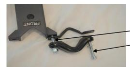
To fit the seat, all you do is loosen the front bolts, and remove one completely,
