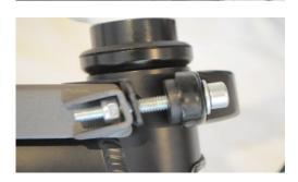
All you then do is tighten the bolts and attach the seat.
